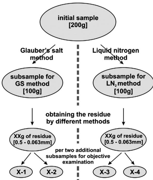
Fig. 1. Step by step experiment for comparing the GS and LN<sub>2</sub> methods.
