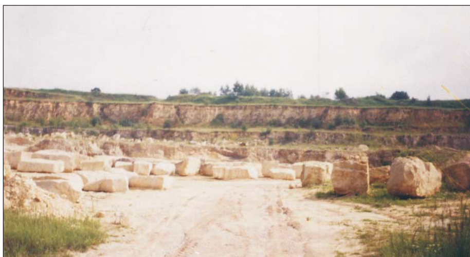
Fig. 1. The quarry in Pińczów with three Badenian organodetrital limestone types; from the bottom upwards: fine-grained, medium-grained, coarse-grained limestones (Photo by A. Chruszcz).
